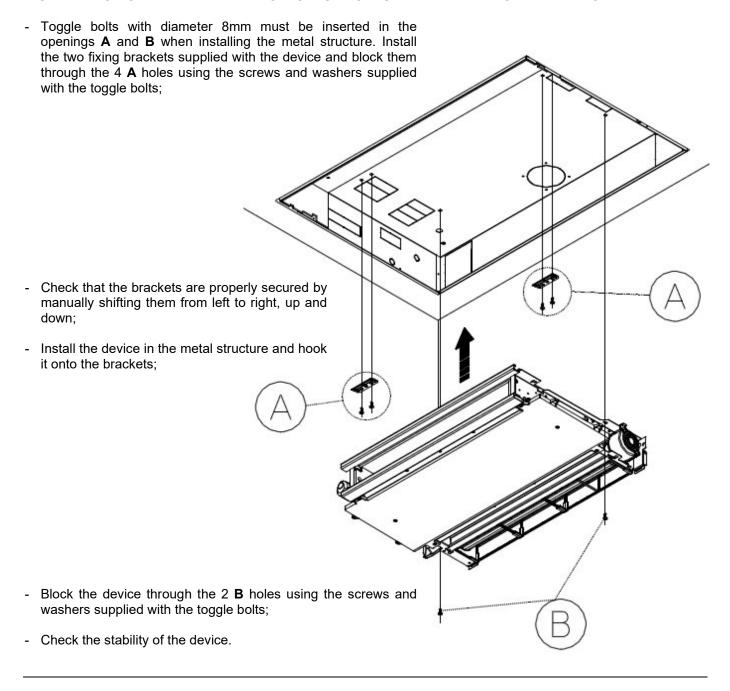
INSTALLATION OF DEVICE IN METAL STRUCTURE SECURED USING ANCHORS DETACHED FROM THE CEILING:
