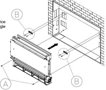
Before assembling the kit, the GRILL, FILTER-STOPPER and FRONT PANEL must be removed by unscrewing the 6 fixing screws in the lower part of the FRONT PANEL.
