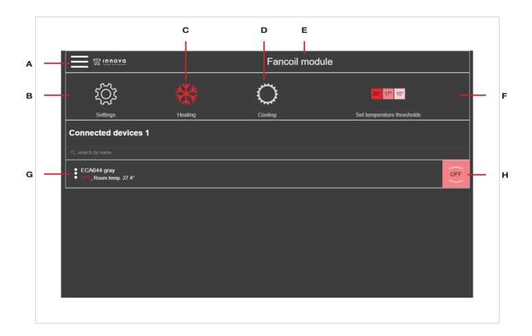
lacktriangle The setpoint displayed in the tile "H " in winter can be subjected to the action of the climatic adjustment, calculated according to the external temperature and may be different from that set in the programming page
