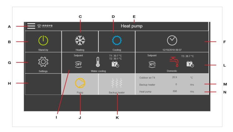
▲ Setpoint displayed on the tile "I" in winter can be subjected to the action of the climatic adjustment,
