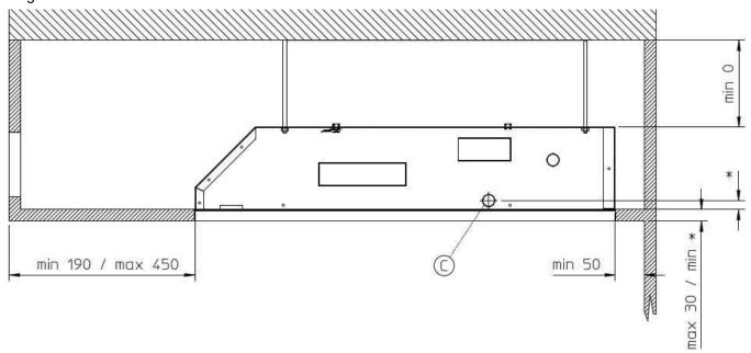
\* If the cooler-convector installed in the metal structure is used to cool rooms, the thickness of the plasterboard must remain completely below the edge of the metal structure in order that piping for the discharge of condensation (outlet hole **C**) can be sufficiently inclined.
