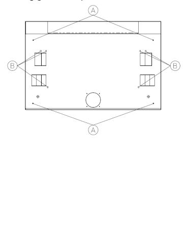
Then install the supporting brackets and the built-in version of the device (securing it through the 6 "B" holes, using the screws and washers supplied with the toggle bolts), install one of the TELESCOPIC AIR OUTLET DUCT kits DB0160/DB0164 and an EXTERIOR PANEL KIT FOR BUILT-IN CEILING INSTALLATION LC0618/LC0622, in accordance with the specific instructions contained in the kit itself.
