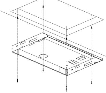
Then install the supporting brackets and the built-in version of the device (securing it through the 6 "B" holes, using the screws and washers supplied with the toggle bolts) and an EXTERIOR PANEL KIT FOR BUILT-IN INSTALLATION LC0578/LC0582, in accordance with the specific instructions contained in the kit itself.
